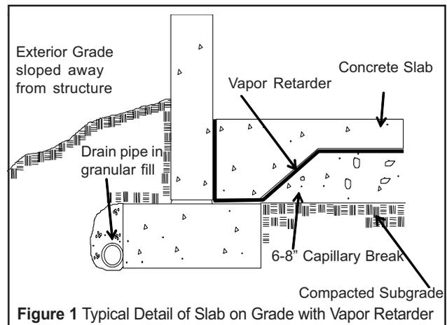
ten are converted to other uses and then moisture-sensitive flooring is installed. Such “adaptive re-use” cannot be predicted during design and construction of a new building. Therefore, it is sensible planning to include a vapor retarder under every interior floor slab in every building. Vapor retarders are generally not necessary when placing exterior slabs on grade.
